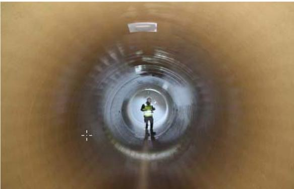
The pipes made of glass fibre reinforced plastic are the basic material for the manufacture of water storage tanks and complex modules for drinking water storage.
